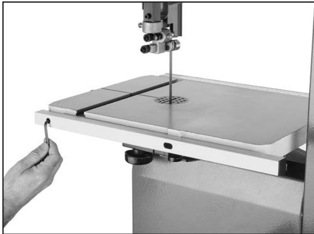
Figure 16. Rear rail installed.
